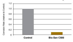
Corrosion Rate at 50 ppm H<sub>2</sub>S
