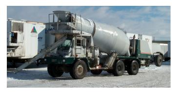
Cummins L-10-300 Engines, Allison HT-740 Automatic Transmissions, Oshkosh 21,000 lb driving front axle, Rockwell RT-46-160P, 46,000 lb tandem axles, 32' Illinois Spec Bridge Formula "Load Span" with 72" spread tandem axles, 11 yard mixers with Hydraulic Power Chutes, Drum Start/Stop, 150 gallon aluminum Water Tanks, Air Flip Hoppers, Piggyback Chute Cylinder, ZF Drum Drive, High Back Cloth Seats
