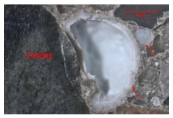
Fig. 5: Alkali-silica gel (arrows) in voids near reactive gneiss particle.
