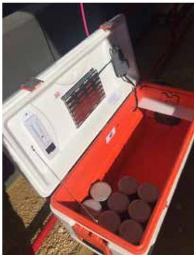
Cylinders cast for the purpose of acceptance testing should be cured via standard curing. Acceptance testing is done to check if the concrete meets contract specifications, and it
