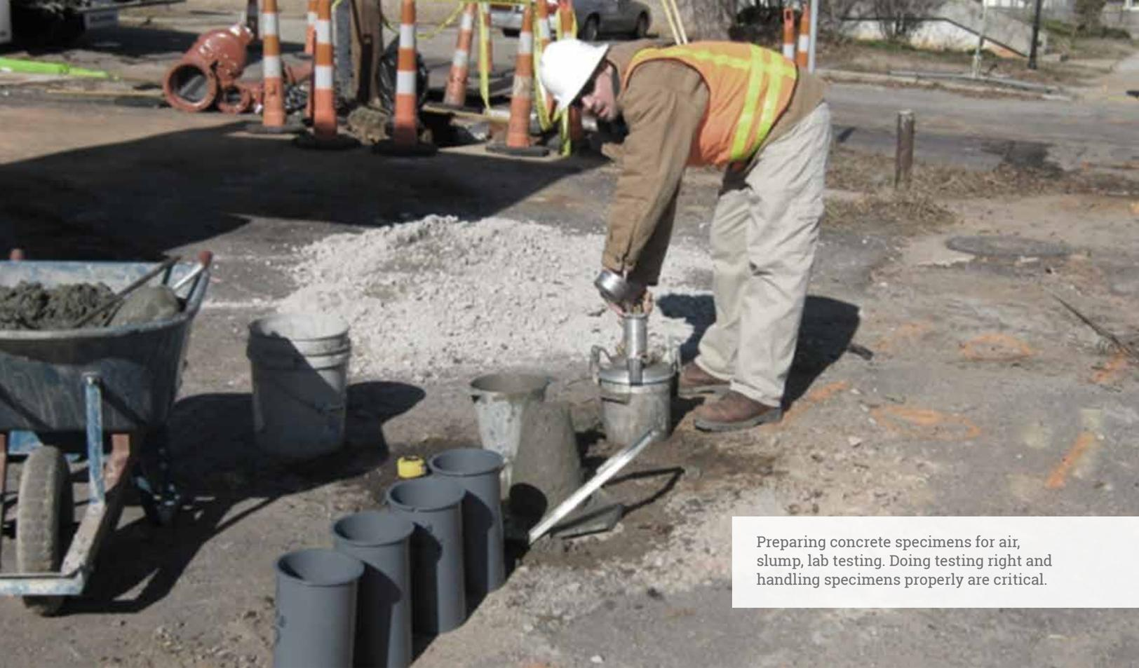
Preparing concrete specimens for air, slump, lab testing. Doing testing right and handling specimens properly are critical.
