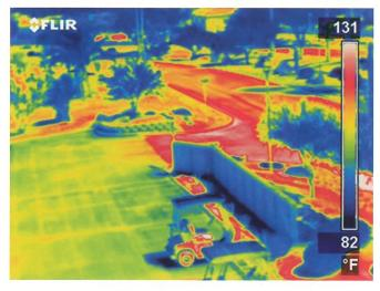
Above are two types of images taken of the same location. In the top photo you see how concrete and asphalt pavements are adjacent. The bottom infrared photo demonstrates the dramatic temperature differences of the two pavements. UTW is much cooler. Photos courtesy of American Concrete Pavement Association.
