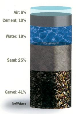
Figure 1: The primary ingredients of concretecrushed stone or gravel, sand and water-account for approximately 90% of the volume of the mixture and are plentiful in most locations. Cement, which accounts for most of the rest of the mixture, is usually produced and available regionally as well. Image courtesy of the National Ready Mixed Concrete Association.
